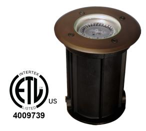
The Cayman well light has an easily adjustable gimbal mechanism that allows precise aiming of the lamp for angled uplighting. Cast brass faceplate with a gasketed heavy-duty composite body. Perfect for spotlighting signs and statuary, as well as for dramatic effects of tree shadows projected against walls.
