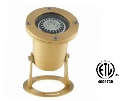
The heavy duty Neptune underwater light is cast from solid brass. The locking shroud features an industrial strength gasket to ensure ultimate protection from water damage while being completely submerged to a maximum depth of 6 ft. Numerous MR16 LED lamp options with various light qualities.
